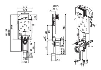
h (height) indicates the drift axis from the completed floor and it is approximately 320 mm. However the absolute measurement should be adjusted in accordance with the drift of the closet to be used.
