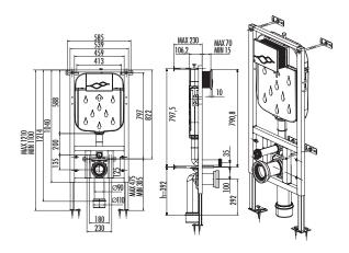
h (height) indicates the drift axis from the completed floor and it is approximately 320 mm. However the absolute measurement should be adjusted in accordance with the drift of the closet to be used.
